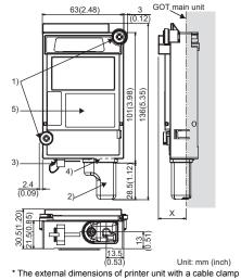
and connector holder attached is shown above
